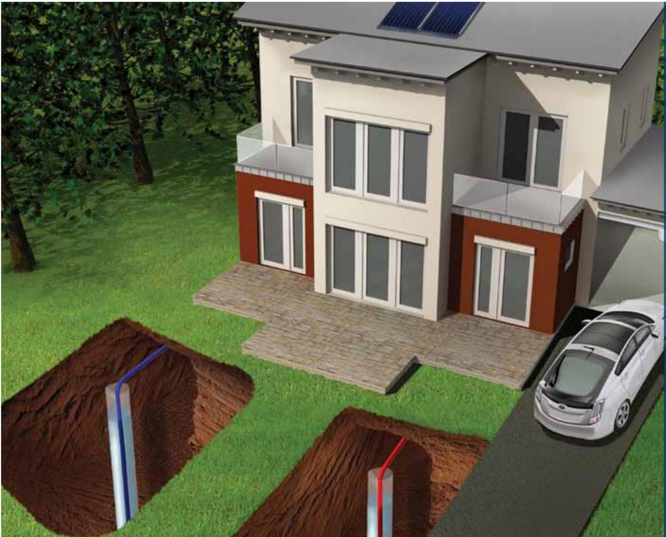
This type of design is only possible if there is sufficient ground water available in a well, a lake or river in the area. The water must be of good quality. Local codes may limit the use of this system in certain areas. The system is open which means that water is pumped directly into the geothermal unit and then discharged either into a return well or a body of water. The water quality remains unaffected.
